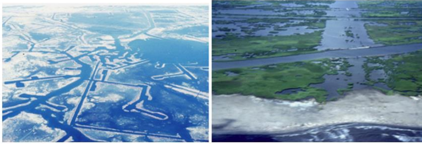
Figure 14 Landscapes of mineral extraction, Louisiana. Left shows how canal construction for petroleum extraction in coastal wetlands has contributed to large amounts of land loss. Right shows that canal construction normal to the shoreline makes barrier shorelines more prone to overwash, whereas canal construction parallel to shoreline acts as a sink for sediment in landward-migrating barrier beaches (photo credits: J. Mossa).
