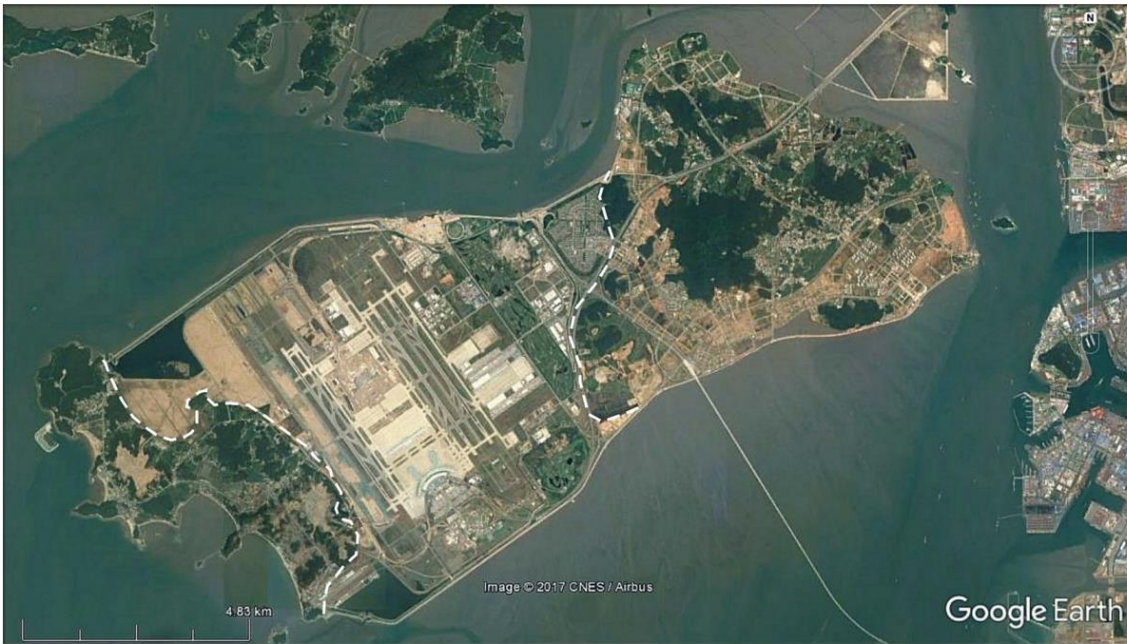
FIGURE 6.3 Incheon International Airport in Seoul occupies most of the reclaimed tidal flats between two already existing islands. Broken line indicates outlines of the islands before reclamation. Source: © Google, CNES/Airbus.
